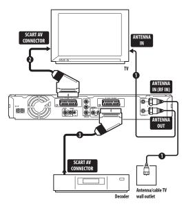
**1 Connect RF antenna cables as shown.** This enables you to watch and record TV channels.
